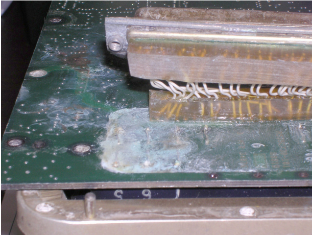
Figure 3-29. Corroded Circuit Card
