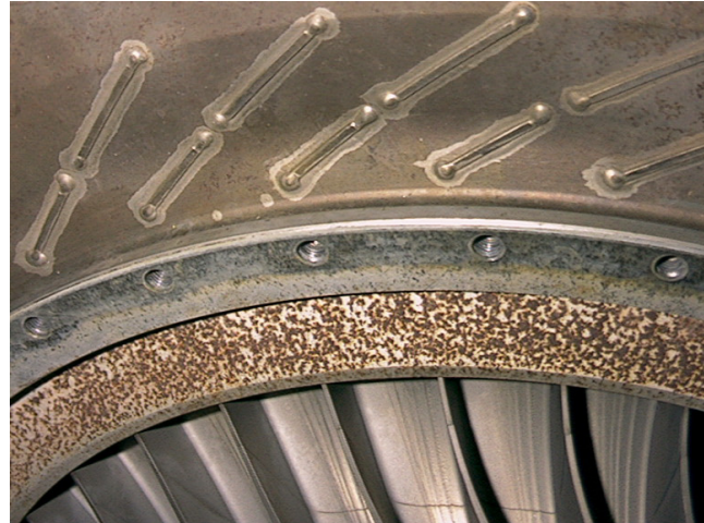
Figure 3-22. Hot Corrosion on Engine Components
