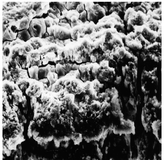
Figure 3-12. Scanning Electron Micrograph of a Corroding Aluminum Surface
