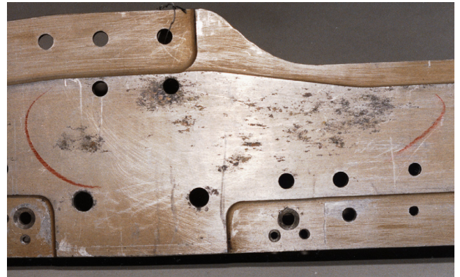
Figure 3-10. Pitting of an Aluminum Wing Assembly
