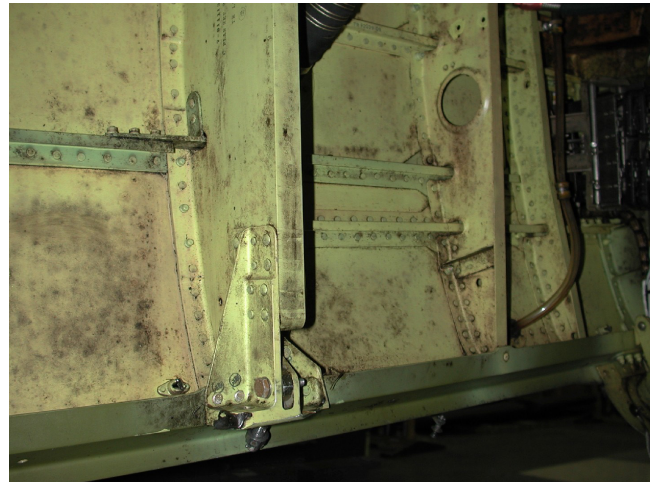
Figure 3-30. Biological Growth on Helicopter Wall
